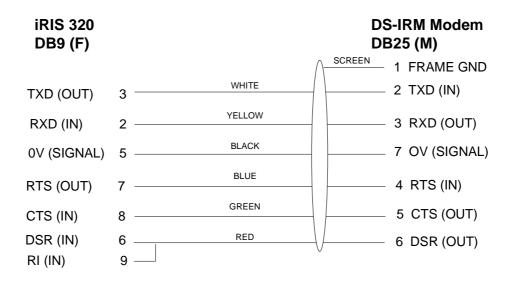
Figure 14 – Typical RS232 / Radio Modem Cable
